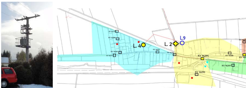
Figure 22: Grid section in accordance with example B4 -pole station and the two substation grids under consideration
