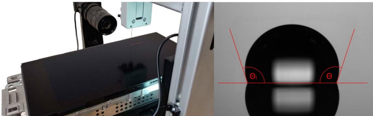
Figure 9 – Contact angle measurement device (SOURCE: Innowep GmbH)
