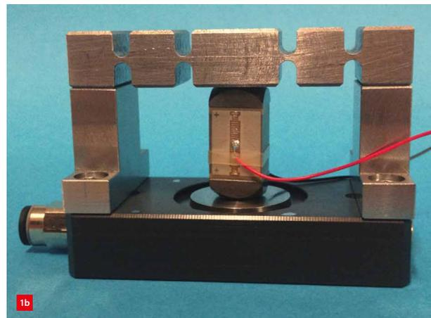
Active thrust pad bearings with PZT/piezo technology. (Courtesy of Politecnico di Torino)
