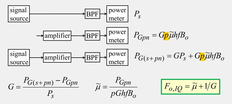
$F_{o,IQ}$  and all other optical NF can be determined from simple optical power measurements.
