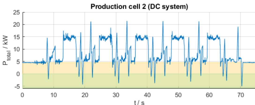
Figure D.42 Traces of power in cell 2 of the HOMAG plant connected to the DC grid without a storage element
