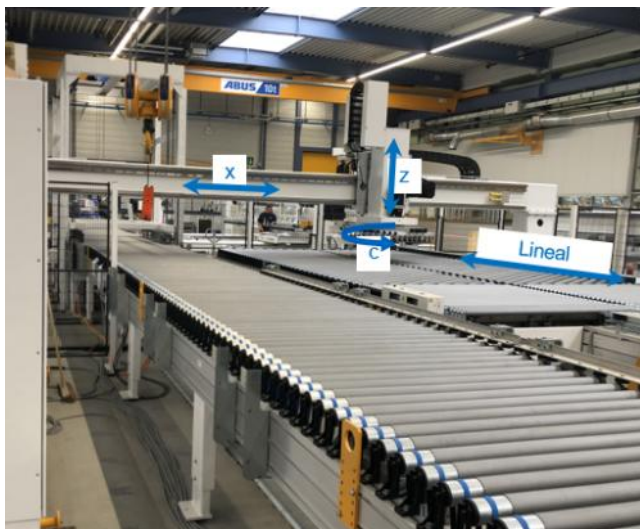
Figure D.43 Handling cell at HOMAG with arrows indicating the axes of motion
