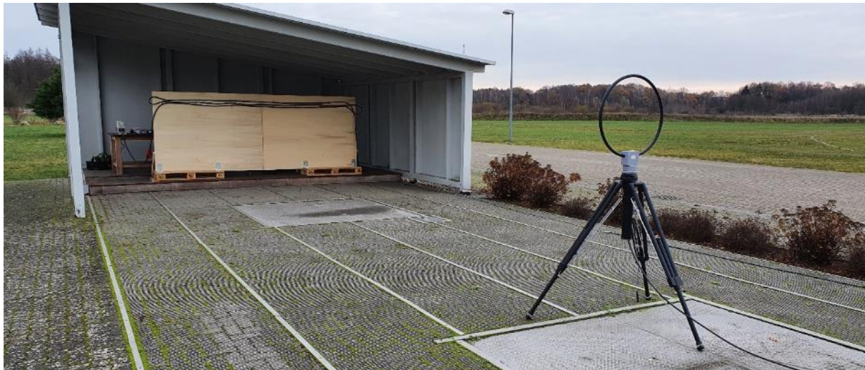
Figure D.13 Outdoor test setup with long supply cable; the frequency converter is on the left and the power supply on the right
